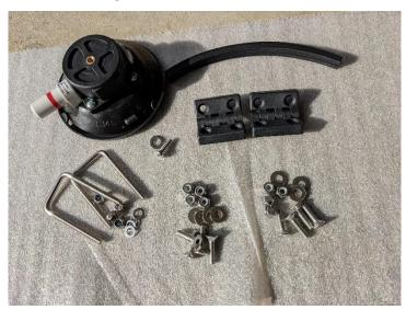
2. Attach rubber to back of bracket where it will hit the Cross Bar Foot. Mount bracket with u bolt M6 washer and stop nut with 10mm wrench or socket
