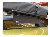
2. Attach hinge to the top of the bracket but don't tighten all the way. With 7/16 wrench or socket and 4 mm hex
